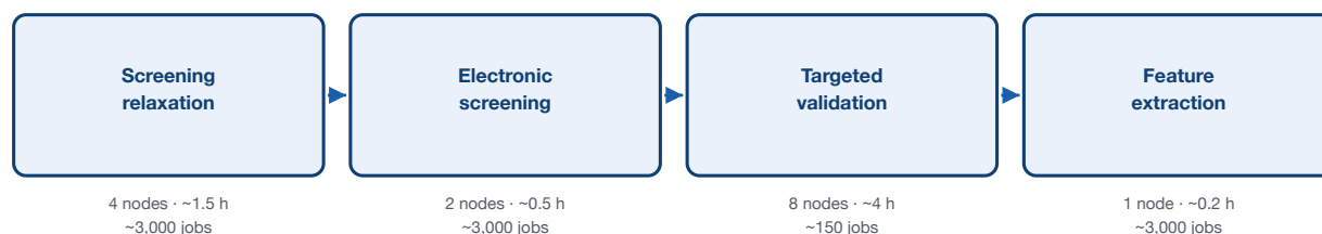
Figure 1. The four-tier compute workflow, with data dependencies flowing left to right — each tier's job count and typical per-job node/wall-time configuration matches Table 2 below.
